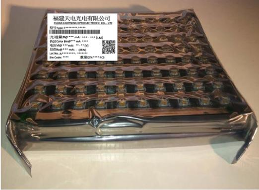
Note: 45 pcs per tray and 5 trays are stacked together to be sealed in an anti-static bag.
